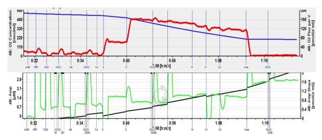
The full experiment showing oxygen-related data on the upper panel and AmR data on the lower one, allowing to correlate respirometric data and  $H_2O_2$  production. The AmR signal was calibrated using the addition of  $H_2O_2$  in the presence of mitochondria but in the absence of external substrate (marks '03' and '04').
