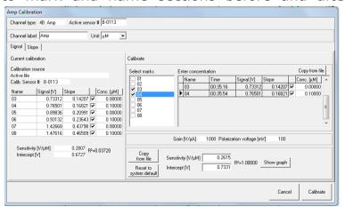
additions, in each case assigning the marks set before and after addition the values '0.000' and '0.100', respectively, taking into account that the immediate conversion of added  $H_2O_2$  by the AmR/HRP assay system will invariantly restore a concentration of  $H_2O_2$  of zero. When all additions
