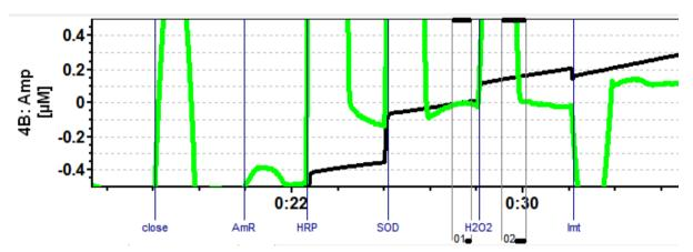
After this calibration step, mitochondria were injected (Imt), followed by another titration of 0.1  $\mu$ M H<sub>2</sub>O<sub>2</sub>. This allows assessment of the optical effect of the sample on fluorescence sensitivity. The fluorescence changes that are subsequently recorded correspond to the apparent H<sub>2</sub>O<sub>2</sub> production by the mitochondria in the absence of external substrates.
