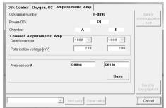
the Amperometric, Amp tab to define the Amp sensor numbers for documentation. Gain for sensor (1000) sets the signal amplification. The light intensities of the are controlled by selecting Polarisation voltage [mV] (100 or 200). The light intensity may be optimized preliminary experiments to obtain a signal
