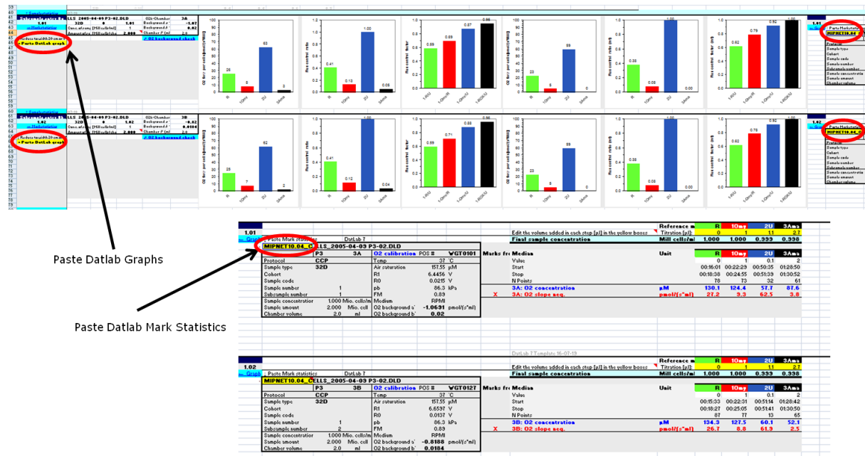
Figure A1. Datlab analysis: Marks Statistics [F2] is copied to clipboard and pasted into the Excel template "SUIT_MiPNet10.04_IntactCells.xlsx" for each chamber. The bar graphs for each individual experiment are then displayed automatically. The corresponding Oxygraph-2k traces (DatLab graphs) for the two chambers are copied to clipboard and pasted into the DatLab-Excel file.
