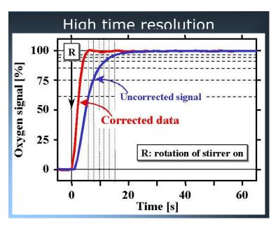
Sensors respond with a time delay to rapid changes of oxygen (uncorrected signal). Is the oxygen sensor sufficiently fast for kinetic studies? DatLab yields the answer, gives the exponential time constant and displays the time-corrected data (modfied after Gnaiger 2001).
