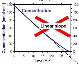
time, flux over and oxygen estimated from the (respiration) is Traditionally, linear slope. sections of the experiment analzed using a ruler on the trace of the chart recorder. With this "eyefitting" technique, traces appear to be more linear than they are. The "linear slope" approach belongs to the past of bioenergetics.
