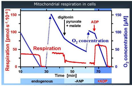
Respiration of intact endothelial cells (endogenous respiration in mitochondrial medium), and after cell membrane permeabilization by digitonin (resting state 2 in the absence of ADP; activated state 3 after addition of ADP). Reoxygenations are simple during the experiment (dotted arrows). DatLab 4 displays on-line oxygen concentration [µM] and oxygen flux (respiration).
