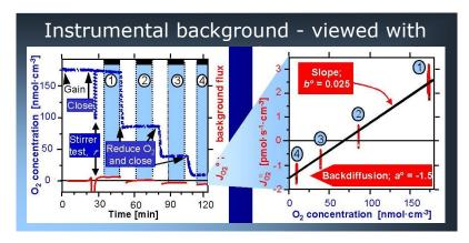
Corrections for instrumental background are an essential standard in high-resolution respirometry, automatically performed by the DatLab software (modified after Gnaiger 2001).
