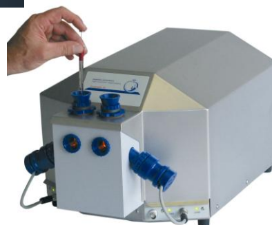
Figure 1. The OROBOROS® Oxygraph. A , window into chamber A; B , glass chamber B; both chambers are housed in a copper block (temperature-regulated and insulated). Peltier thermopiles are in thermal contact between copper block and Peltier heat dissipation plate. Polarographic oxygen sensor (POS) with butyl india rubber sleeve for sealing the POS against the glass chamber.
